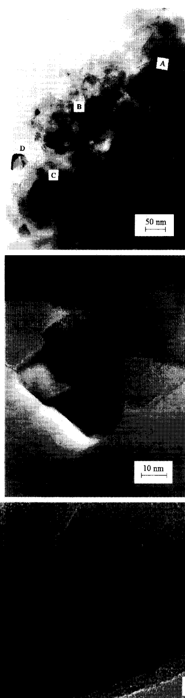
Fig 6. (a) Transmission electron micrograph at low magnification of the product of shock compression; (b) transmission electron micrograph at high magnification of a well-faceted grain of diamond with size in the range 50–100 nm; (c) transmission electron micrograph of a graphitized carbon black particle. The interlayer spacing is around 3.6 Å.
