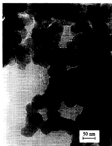
Fig 1. (a) Transmission electron micrograph of carbon black used as starting material. The spherical particles are roughly 40–50 nm in diameter;
